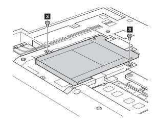
**6** Remove the frame fixing screws **3**.
